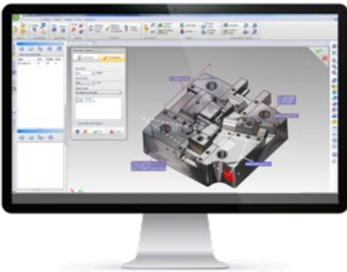
Dimensioning in a component assembly
